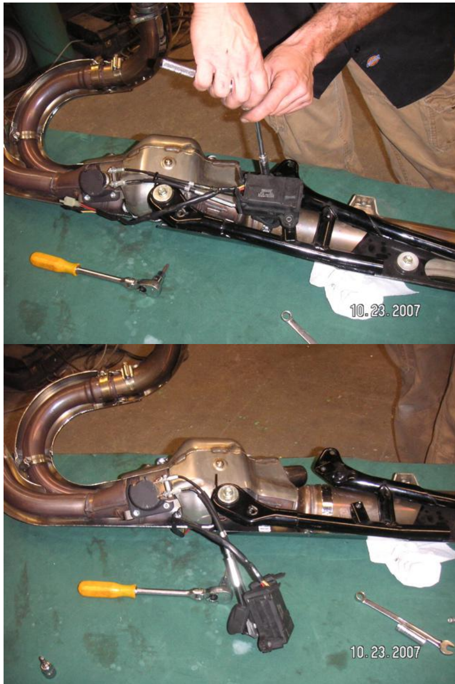
Remove exhaust actuator from support frame. There is no need to disconnect cables.
