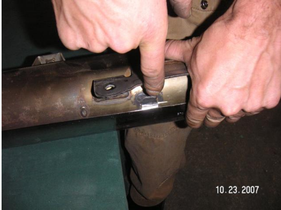
Picture shows weld ground off
