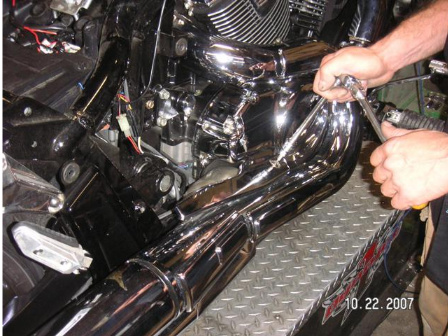
Remove Allen bolt from heat shield
