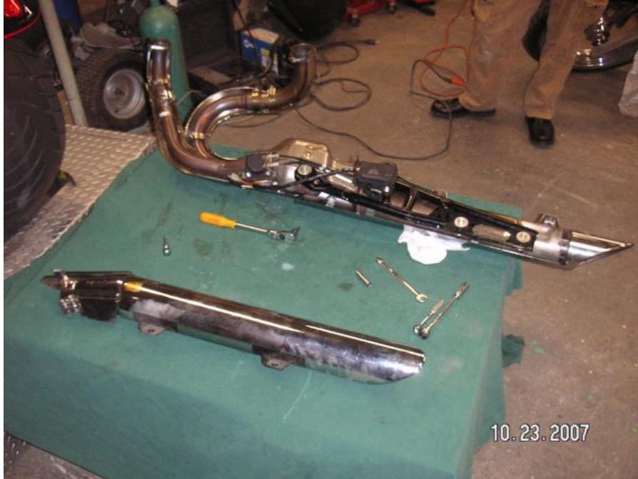
Remove exhaust and place on a covered workbench so you don't scratch any chrome.
