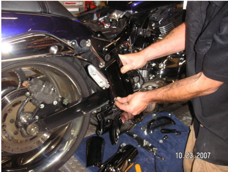
Reinstall Black Trim panel and bolt
