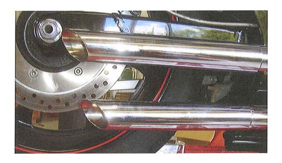
Now that you have the pipes on and roughly aligned, use the support bracket provided to slip over the longer Allen Bolts. You may have to twist the pipe / collar assemblies to get the alignment just right.
