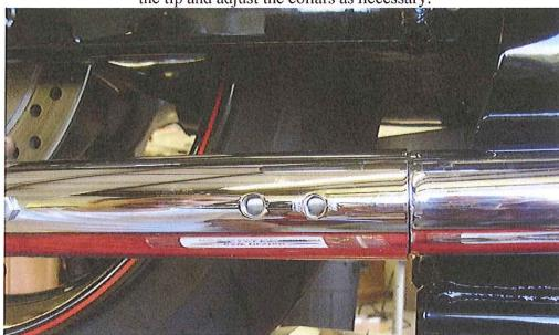
Reinstall the Set Screws through the Tip and into the collar. Make sure The longer screw goes in the forward position. DO NOT TIGHTEN THESE SCREWS!! Leave everything lose for now.
