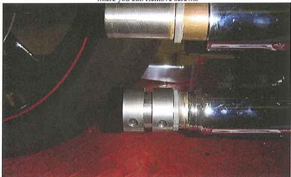
Slip Lower (Shorter) pipe over collars. The (2) holes in the pipe need to line up with the screw holes in the collars. And yes, the slash on the pipe will be facing up. You'll see why in a minute.
