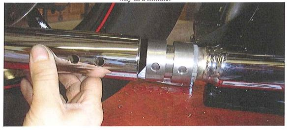
This is how the pipe and collar alignment should look. If it's off a little, slip the Allen wrench you used to remove the bolts into the holes and GENTLY pry them into alignment. If they are off by more than about ½ a hole diameter, you'll need to remove
