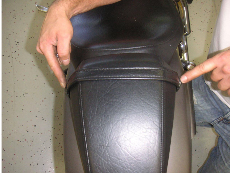
Remove (2) Allen Bolts from Seat Strap.
