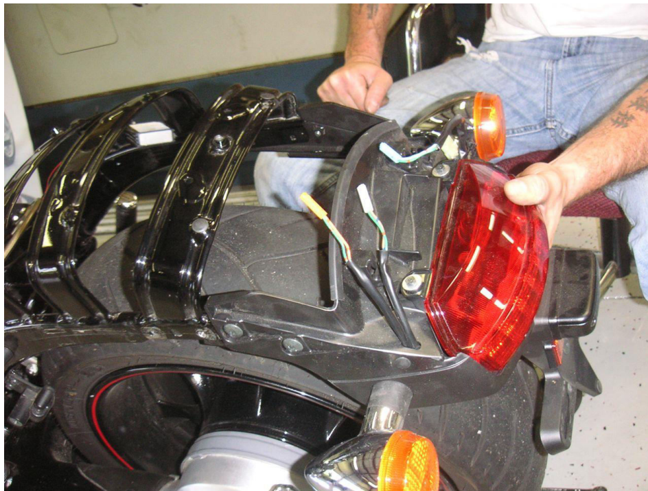
Disconnect (4) Snap connectors from stock Taillight assembly. 3 are clearly shown here. The 4 th is the larger white connector seen in front of right turn signal.
