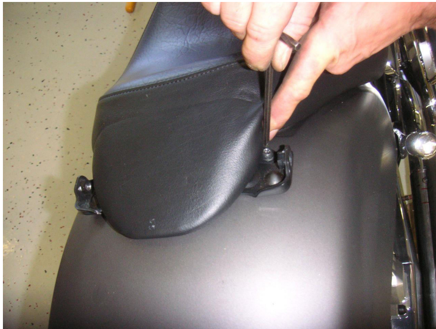
Remove (2) Allen Bolts from back of Rider Seat.
