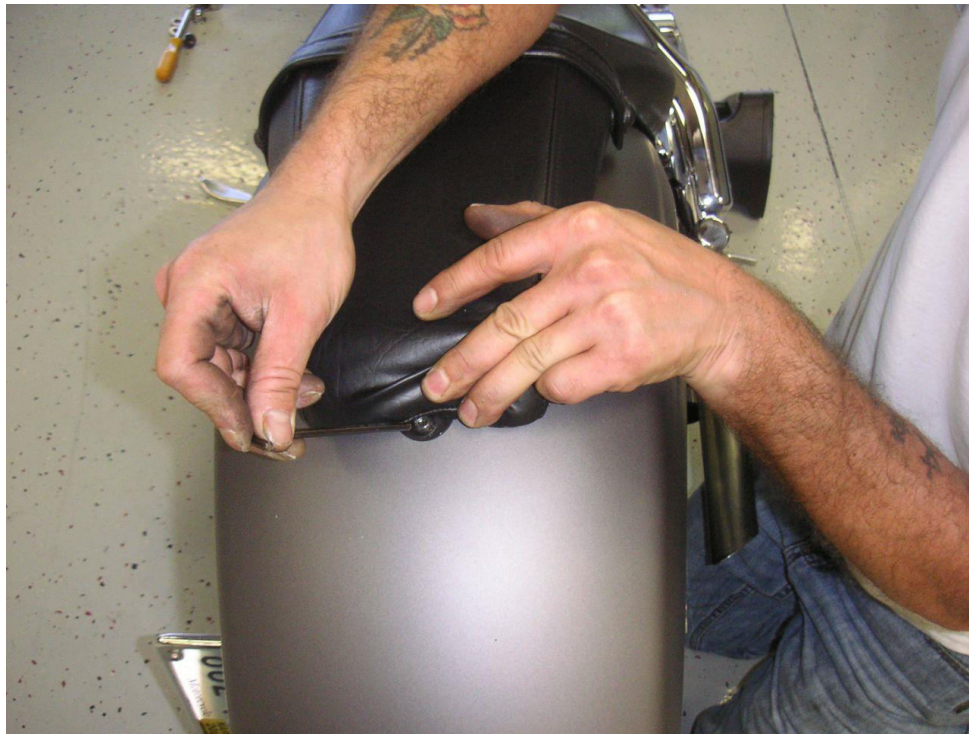
Remove Allen Bolt from underneath of rear of Passenger Seat.
